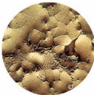
FIGURE 5 A Smooth Surface? If you look at the polished surface of an aluminum alloy under a powerful microscope, you'll find that it is actually quite rough.
