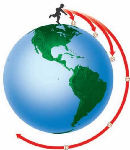
FIGURE 22 Satellite Motion The faster a projectile is thrown, the farther it travels before it hits the ground. A projectile with enough velocity moves in a circular orbit. Interpreting Diagrams How does the direction of gravity compare to the direction of the orbiting projectile's motion at any point?
