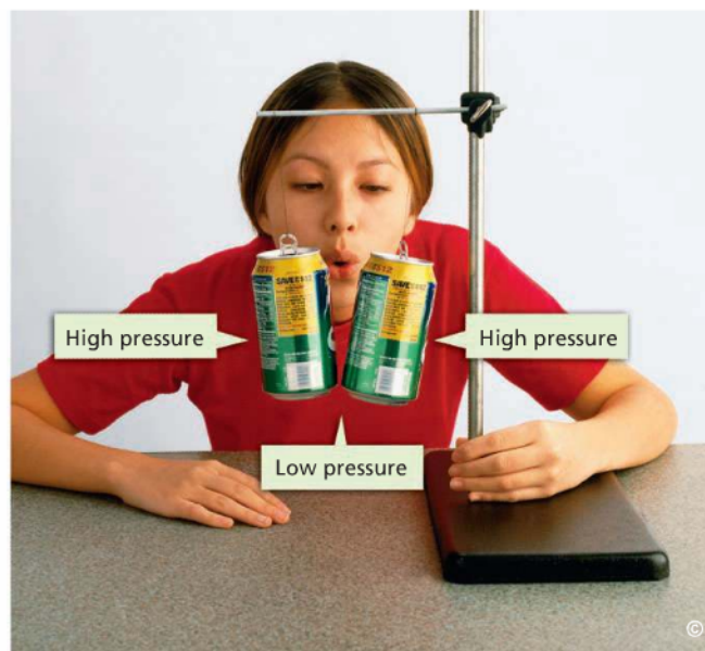
FIGURE 16 Making Air Move Blowing air quickly between two cans lowers the air pressure between them. Higher pressure exerted by the still air to either side pushes the cans toward each other.
