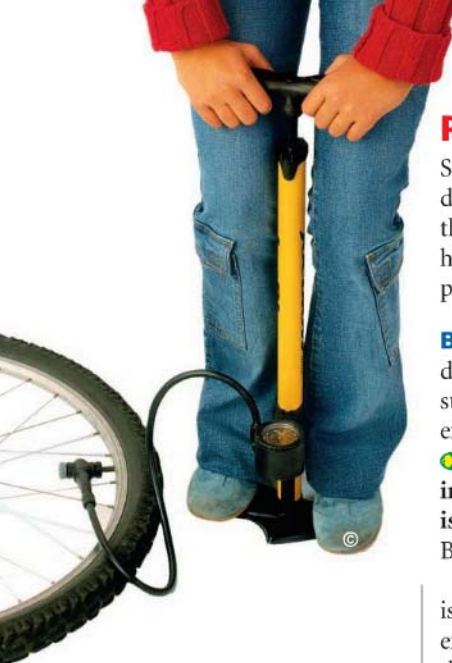
FIGURE 19 Inflating a Tire A bicycle pump makes use of the relationship between the volume and pressure of a gas.
