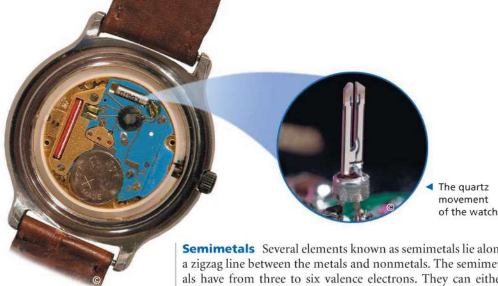
FIGURE 6 A Semimetal at Work This quartz-movement watch keeps time with a small quartz crystal, a compound made of the semimetal silicon and the nonmetal oxygen. The crystal vibrates at about 32,000 vibrations per second when a voltage is applied.
