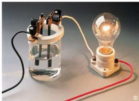
FIGURE 12 Ions in Solution A solution of sodium chloride conducts electric current across the gap between the two black rods of a conductivity tester. As a result, the bulb lights up.
