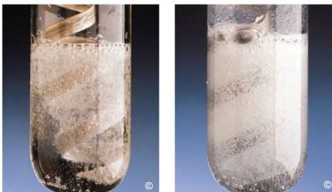
FIGURE 15 Concentration and Reaction Rate Bubbles of hydrogen gas form when magnesium reacts with acid. The solution heats up quickly, indicating that the reaction is exothermic.
