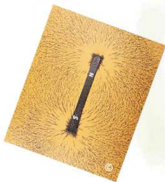
Bar Magnet's Magnetic Field The pattern of iron filings was made by sprinkling them on paper placed under a bar magnet.
