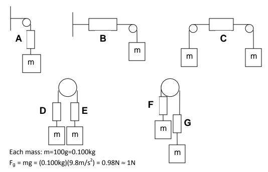
**PREDICT** the reading in Newtons on <u>each of the spring scales</u> shown in the pictures. Remember that these readings indicate the forces that are transmitted by the tensions at various places along the string.
