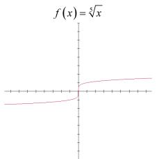
As you can see on the left, the curve is just about the same for a 5<sup>th</sup> root, verses a cubed root. This will be the same case for any radical function where the index is odd. This also means that any radical function where the index is even will look like a normal square root function. The curves of these functions are a little "flatter" than a regular square root or cubed root.
