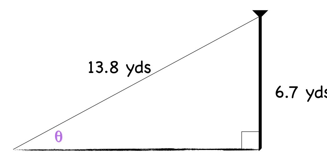
The wire makes an angle of approximately  $29.0^{\circ}$  with the ground.
